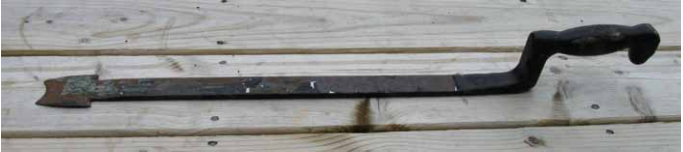
A high quality shingle iron made from carbon steel. A batch of cheap shingle irons sold in Halifax years ago all broke within the first few hours of use.
